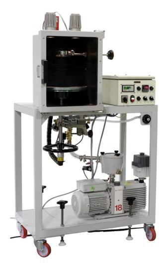
The resin degassing system is fitted with an Edwards E2M18 vacuum pump, complete with exhaust mist filter and inlet trap and solenoid operated air admittance valve.
