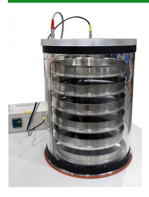
The LyoDry Heated Tray Drying Accessory is one of a range of freeze drying accessories designed for use with LyoDry Benchtop and Midi freeze dryer condensers.
