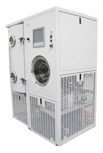
Product heating, drying, end point determination and backfill sequences are all controlled by a central processor unit, allowing complex pressure/temperature profiles to function accurately and reproducibly without operator intervention. In excess of fifty profiles can be stored and retrieved as required.
