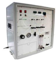
and water respectively. The reaction products are then selectively absorbed into aqueous solutions of hydrogen peroxide and sodium hydroxide, which are then analysed by appropriate radioactive counting techniques. For sampling air, the principle is the same except that a separate air line for oxidation is not required.
