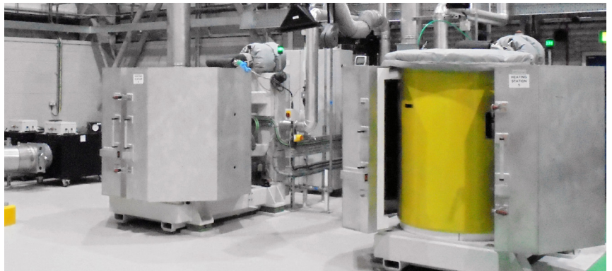
AVDS HEATING STATIONS FOR MOSAIK (CYLINDRICAL) CONTAINER
