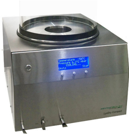
LyoDry Compact benchtop condenser, -55°C OR -85°C
